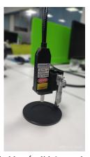
Fig 4 XY probe holder (solid & powder) (optional)
